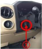
The Battery Boost Switch enables jump-starting the engine from the coach batteries when the engine battery is drained. This switch is located to the left of the steering wheel ① or at the driver's seat below the recline handle ②. If the battery is too low to start the engine, press and hold the Battery Boost/Auxiliary Start switch while turning the ignition switch and release it when the engine starts.
