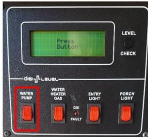
To draw water from the water tank for freshwater supply, the water pump switch needs to be in the ON position. The switch for the water pump is on the battery and tank indicator panel.
